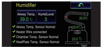
You can check each connection and operation status related to humidifier in one screen at a glance, and you can change settings easily.
