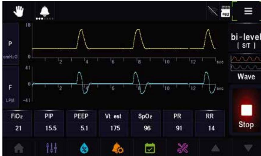
\*Volume guarantee? This function is to convert the target from pressure to volume during inspiration. It can be applied in spontaneous(S), spontaneous / timed(S/T), timed(T) modes, and replaces the inspiration target set value with the tidal volume from the inspiratory positive airway pressure. The provision of tidal volume is limited only by the pressure limit set. Set range: Off, On
