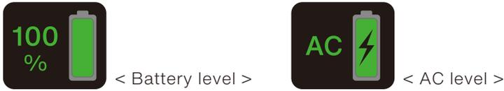
The battery level symbol and percent are checked on the upper right of the LCD. The percent and the gauge inside the battery symbol change according to the remaining battery level. If AC power cord is connected to HFT750, the symbol of the battery level changes to AC power symbol.
